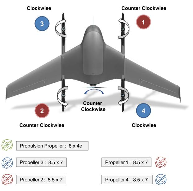
Properly install the quad motor propeller. Please bear in mind the difference rotating direction.
