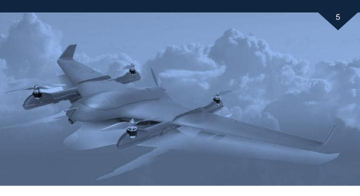
**4SIX+** is a composite vertical take-off and landing VTOL/UAV which is applies fixed wing combined with the quad-rotor complex fixed wing layout, which solves the problem of vertical take-off and landing in a simple and reliable way.
