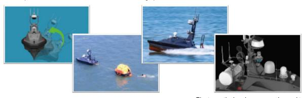
Able to eject a life raft automatically to provide in-time rescue
