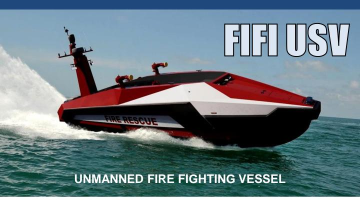
The UFV is a 24/7 autonomous unmanned fire fighting vessel conceived with fast response in mind. With independent berth departure and collision avoidance route navigation, the UFV transits faster and safer to the fire location.
