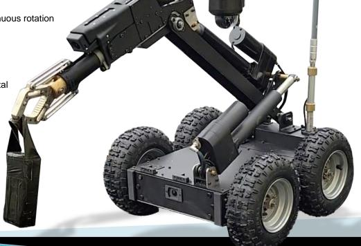
The R-BOT is easy to set up in under 10 minutes, and is controlled by an off-the-shelf Xbox controller. The controller can be plugged directly into the R-BOT or via a laptop that displays the UGV's 4 onboard camera
