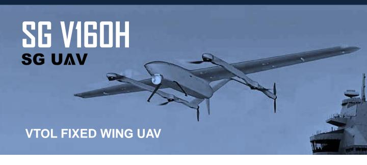
SG V160H is a heavy-duty vertical take-off and landing fixed-wing UAV with a flight time of up to 10 hours and a maximum payload of 15 kg. It provides an excellent solution for cargo transportation and efficient monitoring with a gimbal camera. Its advanced design and features make it an ideal partner for air missions.
