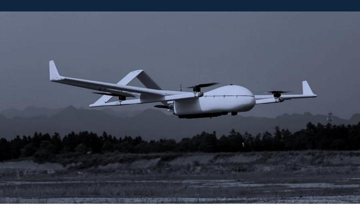
**Outstanding Performance:** 3000m max take off attitude, 5100m max flight ceiling, 840min endurance, exposure delay within 10ms.
