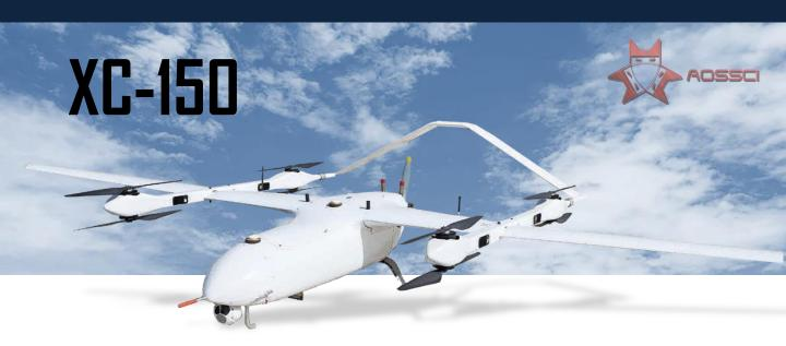
XC-150 is a gasoline electric hybrid VTOL fixed-wing UAS. The entire system adopts a multi-redundancy design to ensure the UAV is highly reliable.
