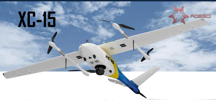
XC-15 is a light and small electric VTOL fixed wing UAV. Its key systems adopt redundancy design to ensure high reliability and safety.
