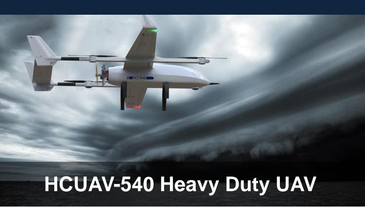
The HCUAV-540 Heavy duty UAV adopts a hybrid electric power system.
