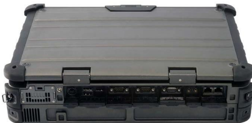
DC Input USB USB + eSATA HDMI Serial Port VGA Audio Output Microphone LAN
