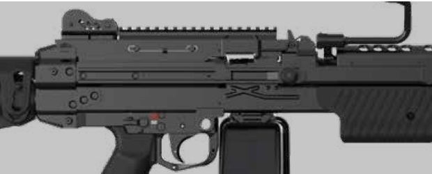
NATO Accessory Rails (STANAG 4694/M1913 Picatinny Rail)
