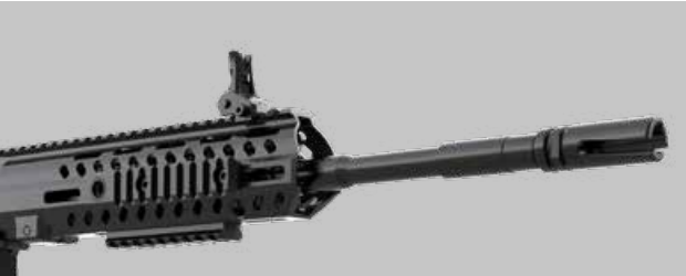
STANAG 4694/ M1913 Picatinny rails on the 4 sides of the handguard / MLOK
