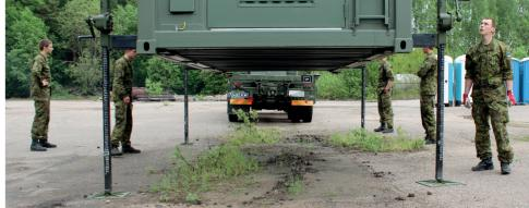
Golden Hour Medical Storage Room is self-sustaining, fully functional in 20 minutes, field hospital warehouse unit, which is capable of preserving up to 10m³ of drugs, blood or any other medical substance.
