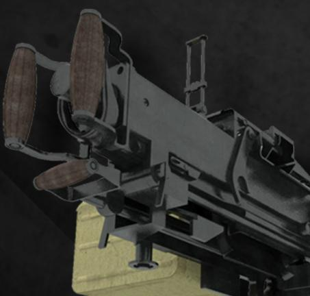
Machine gun is fed from a belt, placed in the ammunition box with the capacity of 60 rounds.
