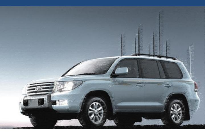
**e) WLAN antenna**. The antenna is a vertical, linearly polarized 4dBi antenna that will be packaged in a standard car roof box.
