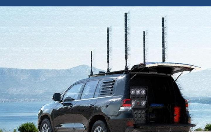
h) 1450 ~ 1925 MHz omnidirectional antenna. The antenna is safely placed in the roof box of the vehicle.
