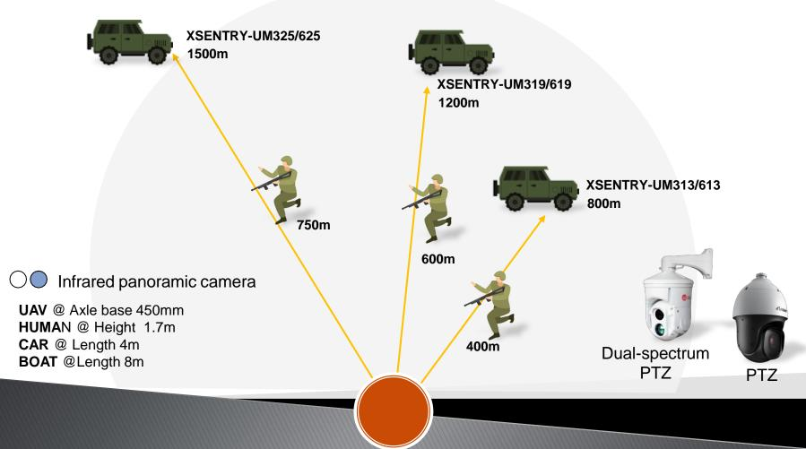
Infrared panoramic camera support tracking the targets and zooming in images of the targets by combining with PTZ, and collect the information related to videos and images and obtain relevant evidence, thus visually presenting the information of targets once the targets are detected.
