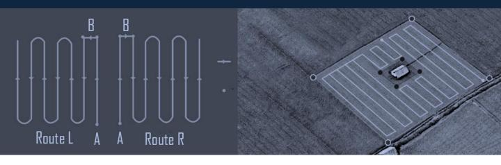
Using GROUND STATION, the user can select the operation area and set operation distance, flight speed, altitude, and other information.
