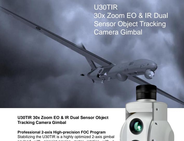
Stabilizing the U30TIR is a highly optimized 2-axis gimbal payload with pinpoint-precise motor rotation with a control accuracy of ±0.01° powered by a dedicated processor. Rather than rely on electrical slip rings, as is common with many gimbals, the U30TIR uses a unique mechanically limited design and concealed wires to ensure more stable data transmission and greater durability.
