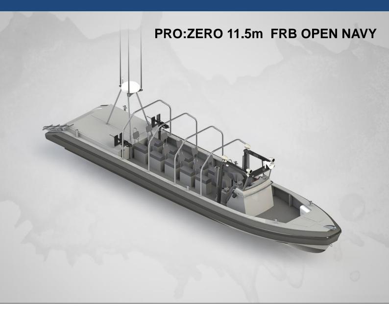
The boat has been designed to meet the specific requirements for navy units to transport up to 10 men or 1,5 tons of load.
