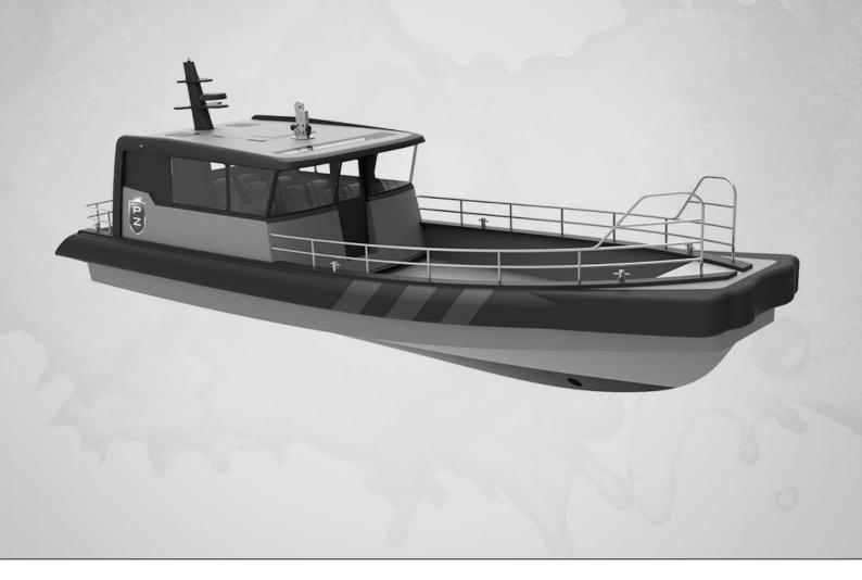
This daughter craft is developed for wind farm service, with a specially designed fender for safe transfers.
