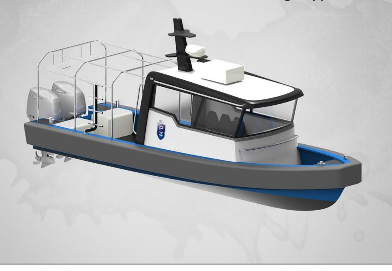
This open boat has is a full covered steering console and a large aft working deck with tent frame.
