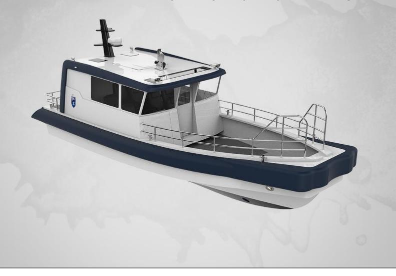
This daughter craft is developed for wind farm service, with a specially designed fender for safe transfers.
