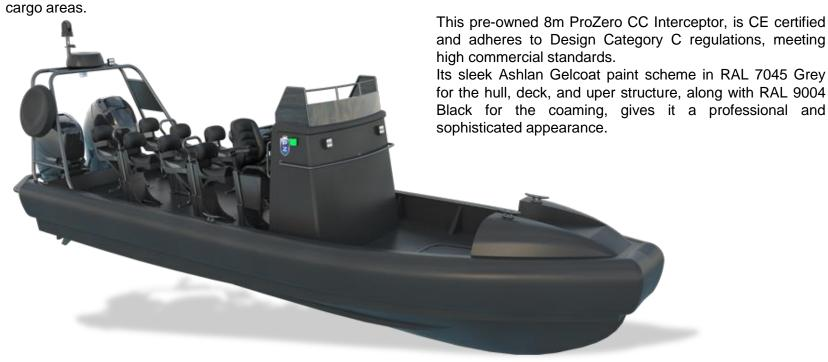
Originally Powered by twin Yamaha 350hp engines (Engines dismounted today) with Sea Star Jackplate HY 4 X-treme and Optimus 360 EST Twin steering systems, this vessel delivers impressive speed and maneuverability.
