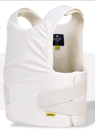
"Titanium SP.3A.301" soft armor panel is designed and developed in order to offer maximum protection at level IIIA according to the NIJ 0101.04 STD. It, also offers protection from multiple threats such as the 7.62x25mm TOKAREV and the 9x18mm Mild Steel Core MAKAROV calibers and protection from sharp edged instruments such as the S1/G blade, with a maximum perforation of less than 16mm at a force of 20Joules according to the NIJ 0115.00 STD.
