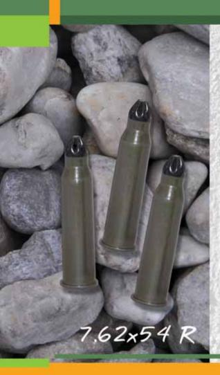
This cartridge is used to imitate the sound of shooting. Compatible with all operational 7.62x54-mm weapons. Firing blank cartridges requires a special plug screwed onto the muzzle to ensure gas pressure sufficient to power gas-operated weapons and disintegrate the dummy bullet, and other special devices according to relevant regulations.
