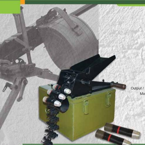
Manually operated Linking Machine is intended for linking 30x29 mm grenades for AGS-17, AGS-30 and ARCUS 17AGL. The machine may be mounted on its packing or on the table.
