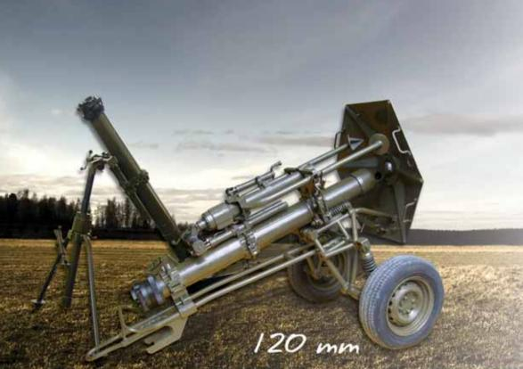
An ideal means against enemy personnel and a battalion level support. The weapon is muzzle loaded and has a classic mortar design with a smooth barrel and a double loading safety device.
