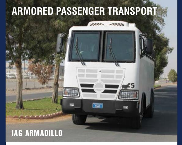
Based on a heavy duty truck chassis, the Armadillo is designed by IAG from the ground up as a large size armored transport bus, capable of carrying 26 passengers and up. Available as a 4x2 or 4x4 and driven by a powerful diesel engine, the Armadillo offers unparalleled level of comfort and protection.
