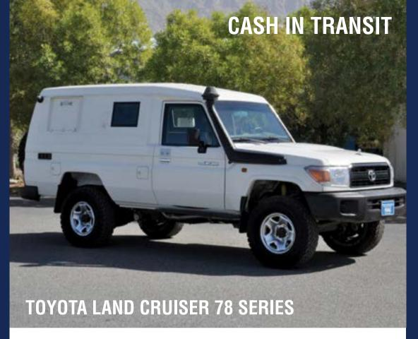
This versatile truck can be used for many applications from low-profile personal protection to a Cash In-Transit vehicle. With a discrete appearance, this CIT is ideal for clients looking to transport money or valuables without attracting attention. The vehicle's high payload capacity makes it suitable to cope with the added weight of the ballistic materials and its day-to-day functions.
