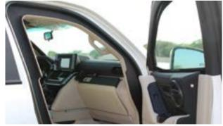
**D00R OVERLAP:** all door apertures in every IAG vehicle is protected with 360 degree, full door overlap.
