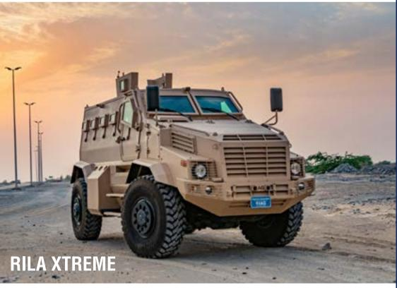
The RILA Xtreme MRAP is equipped with a Cummins diesel engine offering 370HP and Allison 6-speed automatic transmission, 24V electrical system, CCTV, communication equipment and automatic central tire inflation system (CTIS). The independent suspension system provides this vehicle with unparalleled manoeuvrability and off-road capability.
