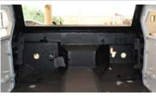
SMARTARMOR™ FIREWALL design with minimal number of pieces, derived from our BRV2009 VR7 certified vehicle, this firewall design provides protection against both ballistic and blast attacks.
