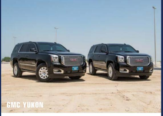
The GMC Yukon is a versatile vehicle suitable for a wide range of applications ranging from law enforcement to personal protection. This spacious vehicle is able to support a high level of armoring up to CEN B6/NIJ III while providing a seating capacity of up to 8 people.
