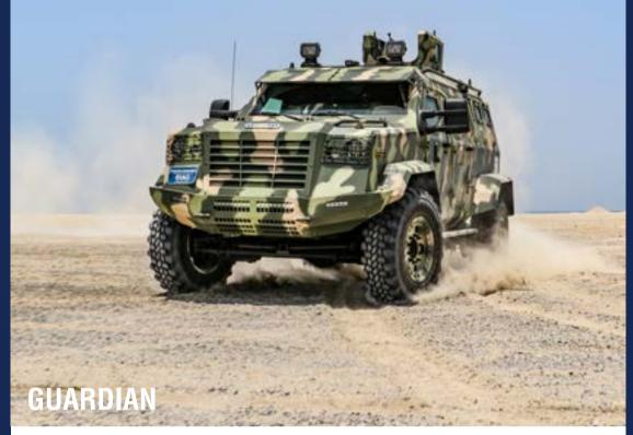
The Guardian APC is IAG's response to the needs of any modern military. Available in LHD and RHD and both 4x4 and 6x6 drivetrains, the Guardian is IAG's flagship APC and offers many different configurations from tavtical ambulance to a 12 person troop carrier. Its level of protection can be taken from the standard CEN B6 up to STANAG Level III.
