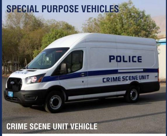
IAG's Crime Scene Unit vehicle can be designed and customized to the specific requirements respective to each department's needs. This vehicle is intended to respond to any crime scene and is equipped with a variety of forensic, laboratory equipment and secured storage for samples and bagged evidence.
