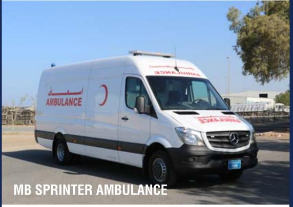
The Mercedes Benz Sprinter is commonly used as a chassis for ambulance conversion around the world. The Sprinter can be outfitted with armoring in addition to the full range of medical equipment, transforming into an armored ambulance suitable for urban operations. Oxygen supply, ceiling mounted IV hooks and Sphygmomanometer are some of the standard equipment in this vehicle manufactured by IAG.
