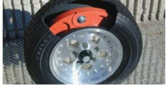
**TIRE, WHEEL AND RUNFLAT ASSEMBLY:** Each armored vehicle comes equipped with certified runflats and heavy duty wheels and tires rated for the after armoring GVWR to ensure optimal performance.
