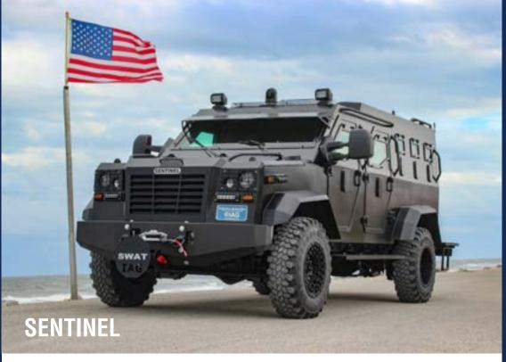
The IAG armored Sentinel Tactical Response Vehicle is based on Ford's heavy duty F550 chassis. It is designed to transport up to 10 fully geared personnel while offering high payload, and unmatched off-road capability. Ideal for law enforcement and SWAT, the IAG Sentinel is available in several protection levels: CEN B6, B7, NIJ III, IV and up to UL10 (.50cal).
