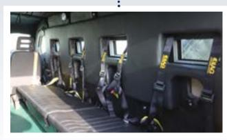
SMARTARMOR™ SINGLE PIECE SIDEWALL DESIGN: the entire length of the vehicle's sidewall is protected with one continuous piece of ballistic steel that integrates all door overlaps and pillars. This provides the highest level of ballistic and blast protection while doubling as a built in roll cage.
