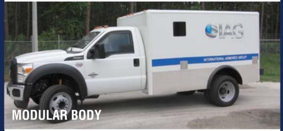
Uniquely designed by IAG, the entire armored box can be unbolted from the vehicle chassis and remounted onto another vehicle frame. Each component within the armored box can also beunbolted and replaced quickly. The Modular Body design is the most customizable CIT truck in the industry.
