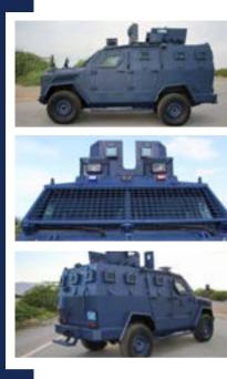
Based on a Toyota Land Cruiser 300 chassis, IAG's JAWS Armored Personnel Carrier can safely transport up to 8 personnel in full combat gear in all road conditions. It is available in both RHD and LHD configurations, with several engine sizes in automatic transmission. Protection levels start at CEN B6, with add-on armor that offers up to level CEN B7.
