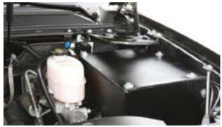
**ENGINE COMPARTMENT PROTECTION:** All armored vehicles come standard with armor protection for both engine side fenders, behind headlights, engine batteries, ECU and brake master cylinder. Full radiator protection is available as an upgrade option.
