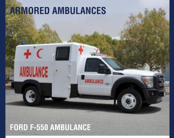
IAG provides a wide selection of armoring and ambulance conversion packages that can be customized to suit specific requirements using the Ford F-550 platform. The vehicle cab is taken apart for full integration of the ballistic armoring. A fully customized armored box available in various sizes is installed at the rear, outfitted with a complete range of medical equipment and medical attendant seating
