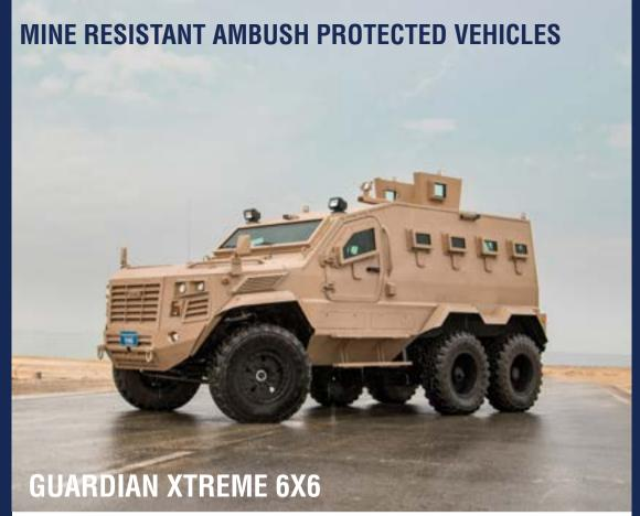
The Guardian Xtreme Mine Resistant Ambush Protected (MRAP) vehicle is designed to meet combat, tactical and surveillance missions and can quickly respond to remote area threats due to its high manoeuvrability. It is available with standard STANAG Level II blast and ballistic protection upgradeable to STANAG Level III using add-on light weight armor. The vehicle has a V-hull shaped floor to provide superior blast protection up to STANAG 2a, 2b and 3a.
