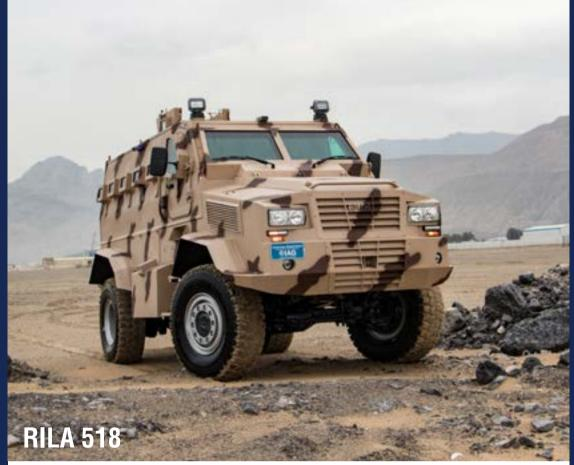
The RILA 518 is the largest MRAP in IAG's portfolio offering ballistic and blast protection up to STANAG level 4. The powerful 12.8L, 380HP diesel engine allows this vehicle to easily travers over any terrain. It can seat up to 12 fully geared personnel situated in blast attenuation seats and is available in  $4\times4$  and  $6\times6$  drivetrain.
