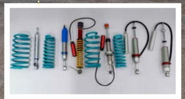
**SUSPENSION ENGINEERING:** Besides replacing the OEM shocks, springs, struts, leafs and/or bushings with stronger, engineered-for-purpose heavy duty components, we have also developed a progressive suspension system that helps evenly distribute the weight of the armored vehicle over many components to ensure the suspension system never fails.
