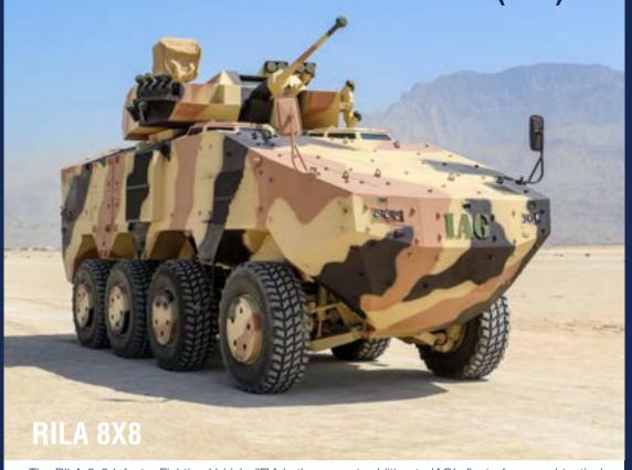
The RILA 8x8 Infantry Fighting Vehicle (IFV) is the newest addition to IAG's fleet of armored tactical vehicles. The RILA 8x8 integrates an armored monocoque hull, offering a low-profile silhouette and large internal volume. The modular design of the RILA 8x8 provides the ability to install a wide range of weapon systems and equipment based on the particular mission requirements.
