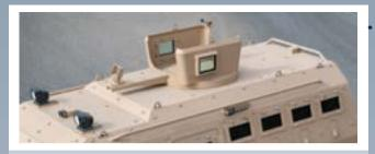
**ROOF PROTECTION:** All armored vehicles produced by IAG come with 90 degrees obliquity ballistic protection in the roof area, as opposed to only 45 degrees obliquity normally found in other armored vehicles. This design offers superior protection against potential attacks.
