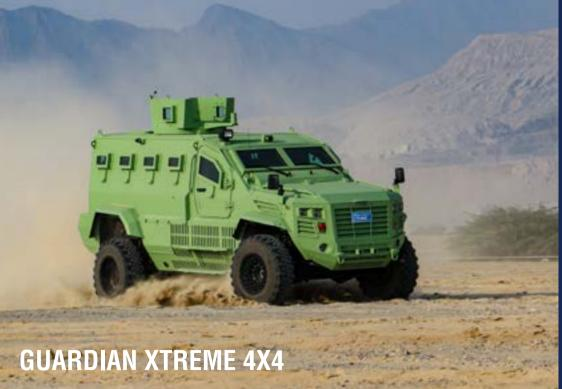
The Guardian Xtreme Mine Resistant Ambush Protected (MRAP) vehicle comes standard with STANAG Level II blast and ballistic protection and can be armored up to STANAG Level III using add-on light weight armor. The vehicle has a V-hull shaped floor to provide superior blast protection up to STANAG 2a, 2b and 3a. It can sit up to 10-12 fully geared infantry personnel.
