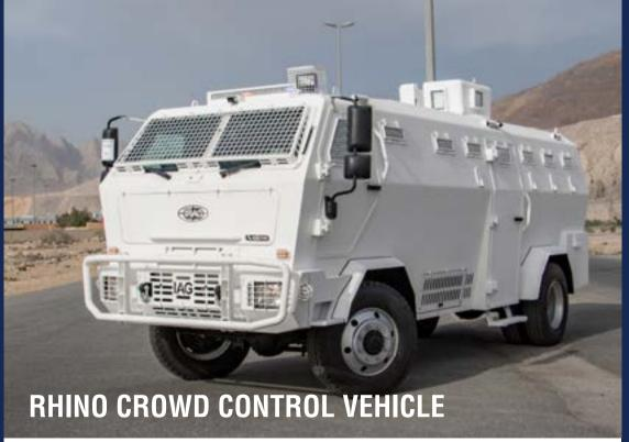
The new addition to the Armored Anti-Riot and Crowd Control Vehicles range, the Rhino is a versatile and multipurpose utility vehicle that can be deployed as a Crowd Control Vehicle or an Armored Personnel Carrier. The Rhino comfortably seats up to 12 fully geared personnel providing five Entry and Exit points for tactical deployment, safety, as well as overall maneuvrability.
