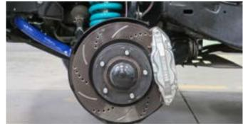
HIGH PERFORMANCE BRAKES: To correct for the new weight distribution and dynamic forces of the armored vehicle, specifically engineered heavy duty brake systems can be installed on every armored vehicle.
