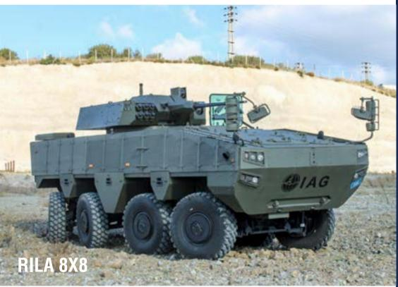
The RILA 8x8 is available in several configurations. This vast range of the 8-wheeled IFV can be armored up to STANAG 4569 LEVEL 4. It is outfitted with a powerful 13.0L diesel engine, producing 550HP and can be driven over 105km/h and maintain a cruising range of 720KM depending on driving conditions. It can seat up to eleven (11) fully geared personnel including the driver and commander. The RILA 8x8 IFV can be fully customized to the requirements of the end user.
