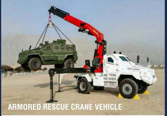
The Armored Rescue Crane Vehicle is capable of carrying out rescue and recovery operations in high risk zones, while providing complete ballistic and blast protection to the operators. It is equipped with a large capacity crane capable of lifting up to 13,000kg (28,600lbs) of weight.
