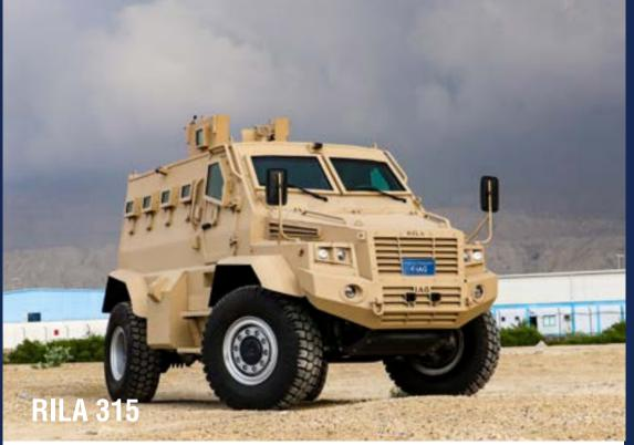
The Rila 315 MRAP offers STANAG level II ballistic protection and up to STANAG level IV blast protection. It is equipped with extreme off-road suspension system, 24V electrical system, CCTV, communication equipment and provides seating for 10 fully geared personnel.
