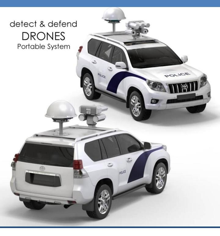
TG-SW-360 UAV detection system includes UAV Monitoring Computer, 360 degree mobile sector antennae and Detection Equipment.
