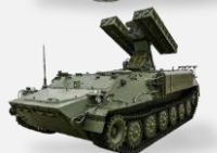
Modernized fighting vehicle of short-range surface-to-air missile system 9K35 "Strela – 10"
