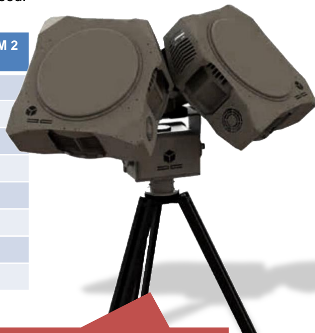
Radar with two antennas covering 180 degrees
