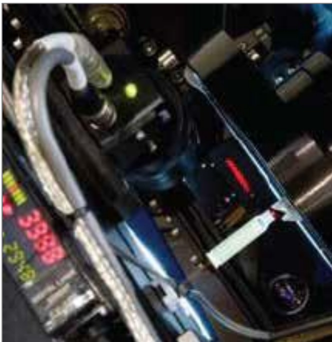
Eight camera inspection system for case defect detection
