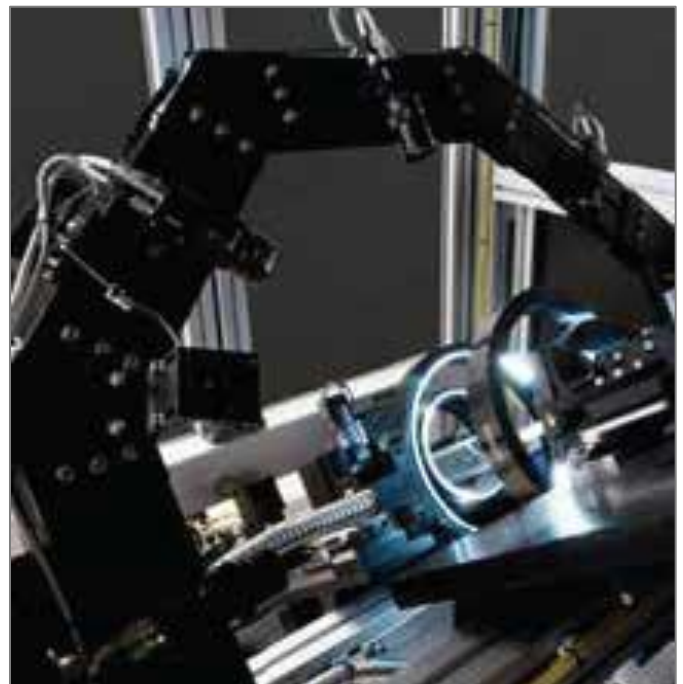
Six high powered LED lighting system for part illumination
